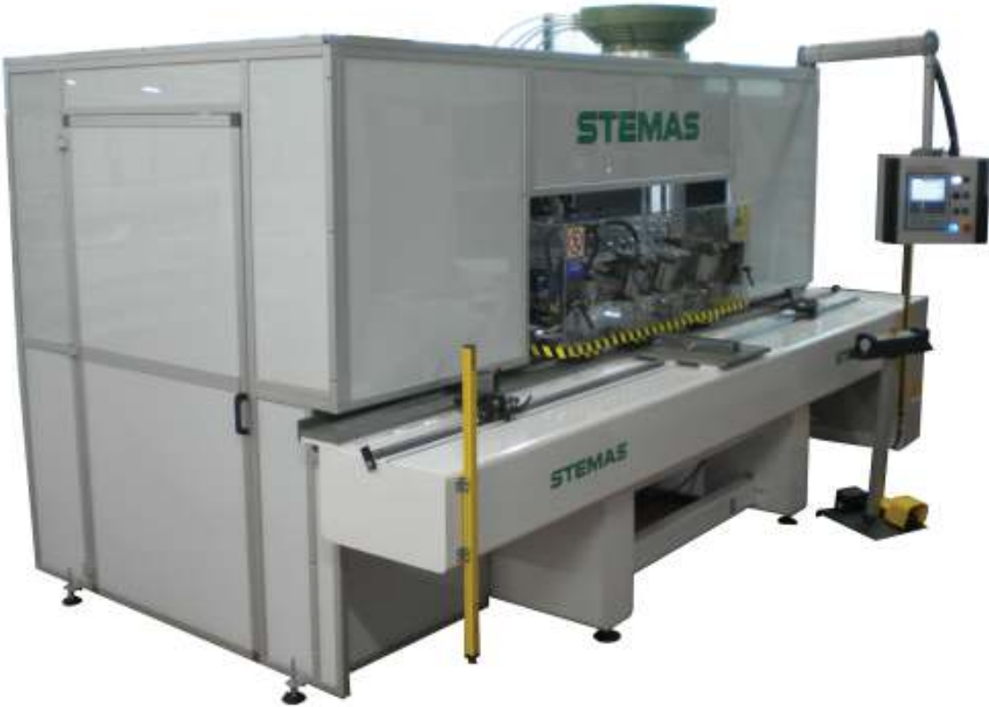
STATIC MACHINERY FOR MILLING, DRILLING AND DOWELING BOTH STILES AND RAILS OF FRENCH-CUT CABINET DOORS
