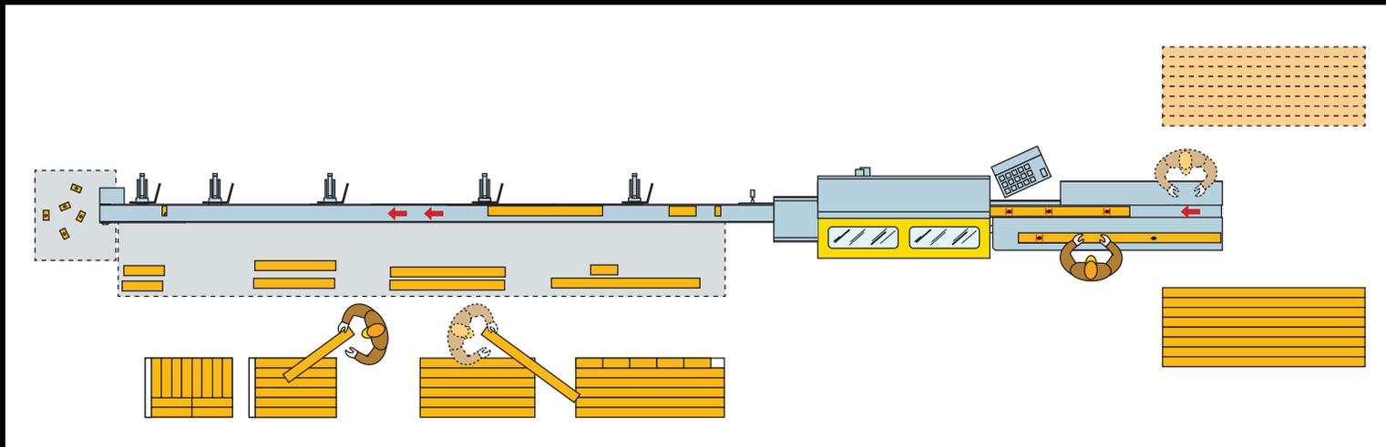
Complete feed system: the dual work piece feed system consists of a high grip feed belt on the underside and cogged rollers on top which adapt perfectly to the wood, thus correctly handling unworked uneven planks.
