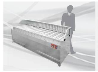
Galvanized sheet workbench with suction from the bottom and from the sides, to carry out sanding operations in total safety thanks to the suction slots on the work top, covered with scratch-resistant felt (optional).
