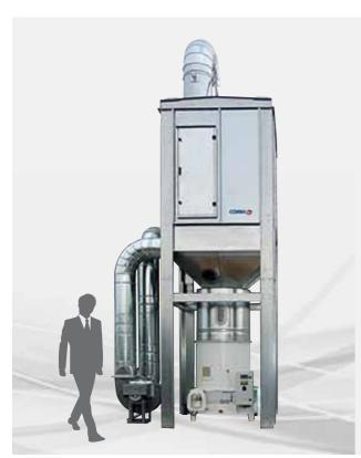
Sleeve filter, with frame or casing in galvanized steel, for indoor installations (where permitted) or outside. Ideal for the filtration of medium-fine particles. Electromechanical **shaking and cleaning system** with eccentric motor. Equipped with large inspection door to facilitate maintenance operations.
