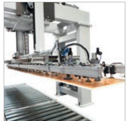
Customising the machine with a suction cup frame enables processing bars for sectioning.
