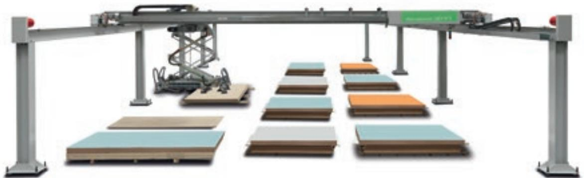
Winstore is an automated magazine for the optimised management of panels for large contract manufacturers, which guarantees production with reduced times and costs. Winstore can be integrated into nesting and sizing cells with a significant increase in productivity.
