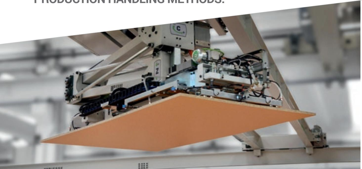
The rotating panel pick-up system and squaring laser photocells optimise the magazine internal area, enabling the perfect alignment of the stack as well as correcting manual loading errors.
