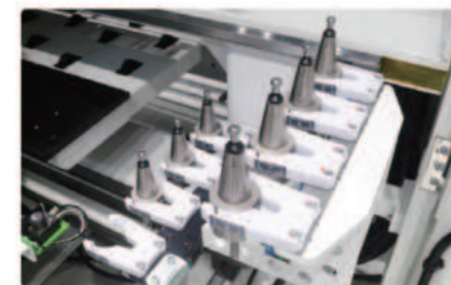
八刀位自动换刀刀库 ATC 8 by servo
