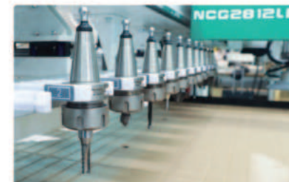
12刀位自动换刀刀库 12-slot line tool changer
