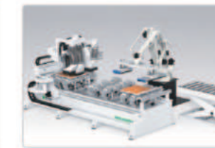
机器人上下料 Loading and unloading by robot
