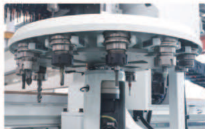
12刀位伺服换刀刀库 ATC 12 by servo
