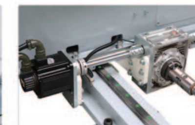
大功率伺服开合装置 High-power servo opening and closing device
