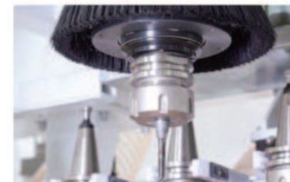
定向吹灰吸尘装置 Directional soot blowing and vacuuming device
