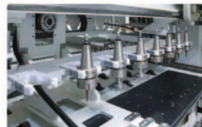
NCB612DPTL配置2组8刀位自动换刀刀库 2 sets 8-slot tool magazine of NCB612DPTL
