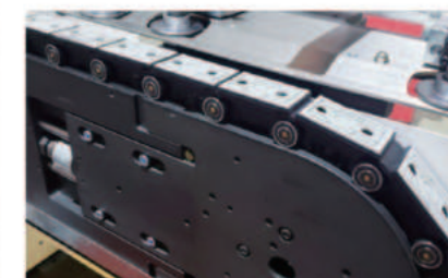
重型坦克链 Heavy-duty tank chain
