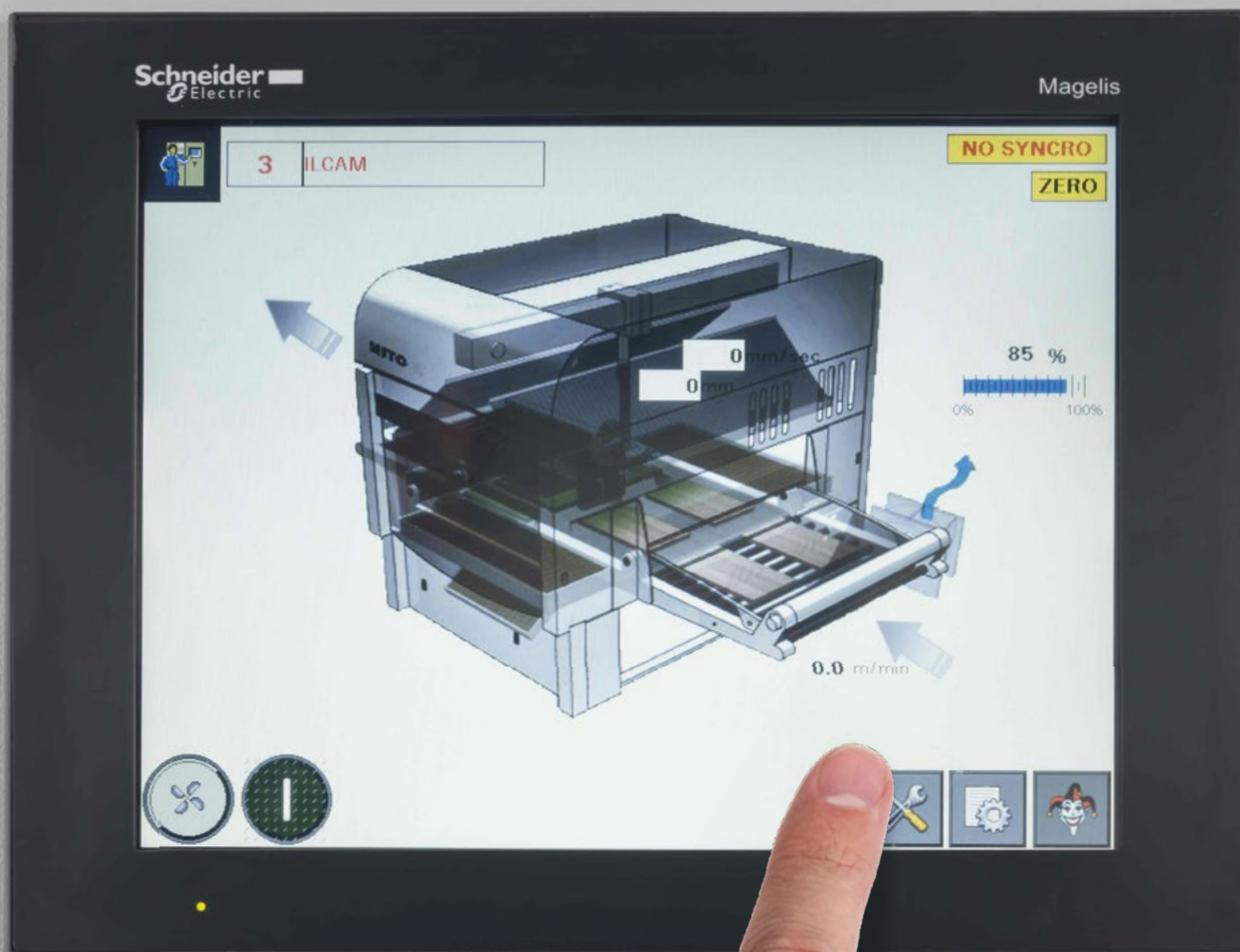
Equipped with PLC and synoptic panel, for userfriendly machine set up.
