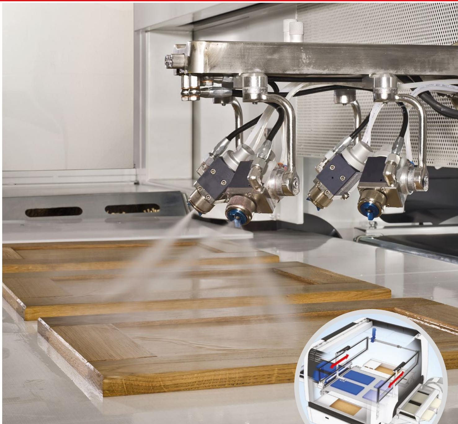
The two spray gun holders are oscillated by means of a brushless motor and toothed belts with separate guides and supports.
