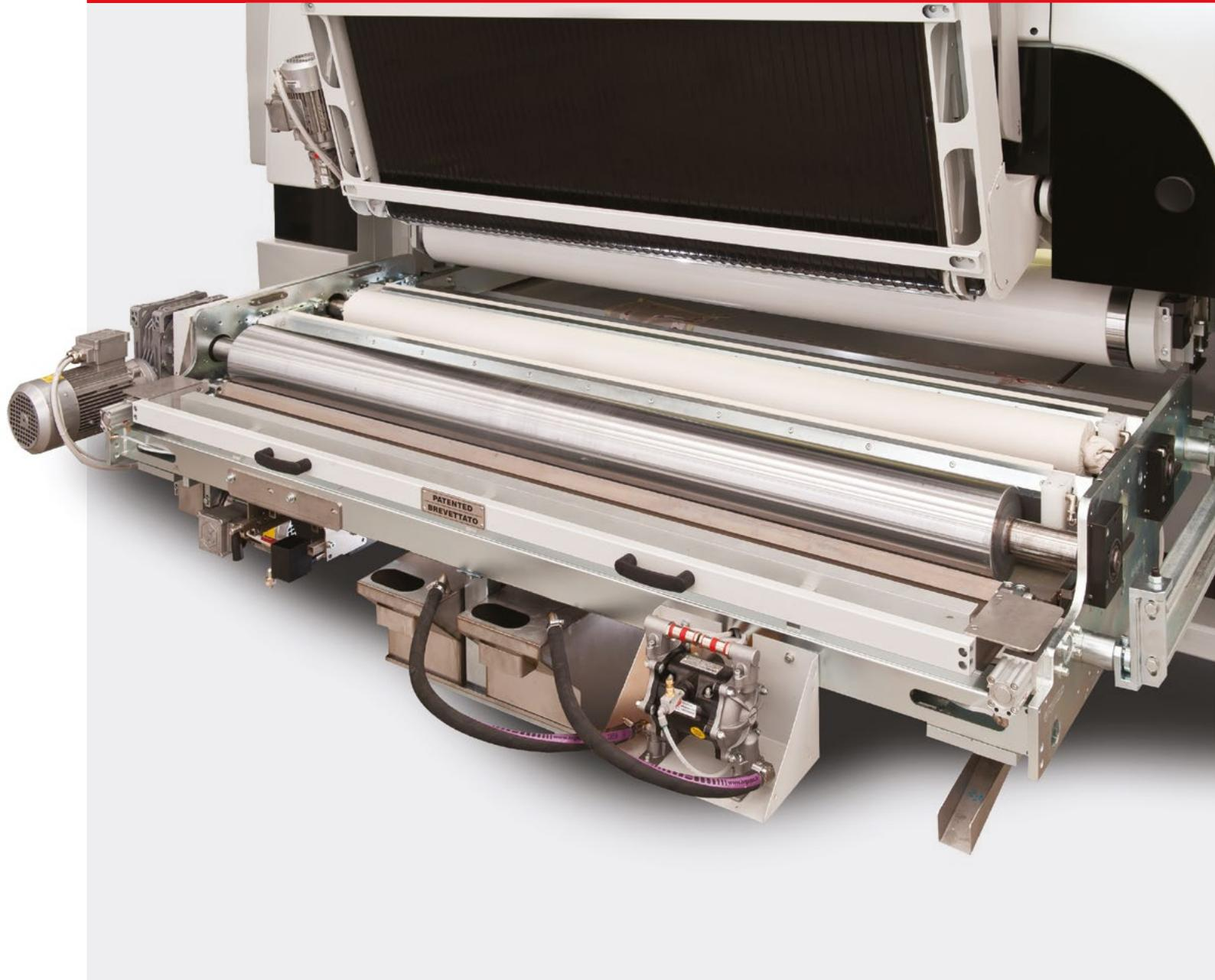
Counter rotating roller removes and recovers lacquer from belt conveyor, while the rest of the system ensures the cleaning of the CFB belt. Cleaning solvent consumption and end-of-shift clean-up time have been reduced to minimum.
