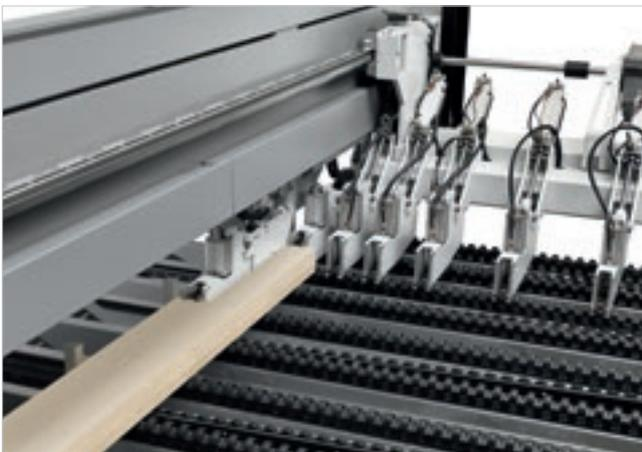
Device for simultaneous execution of staggered cross cuts, made with two completely separate pushers. Each pusher can choose to select one idle slave gripper (not powered) completely independently, based on the strips width to be cut.
