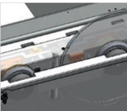
The anti-slide device controls the position and the number of revolutions of the blade, intervening to adjust the advance speed. **Maximum cutting quality, a longer blade lifespan, and reduced maintenance costs.**
