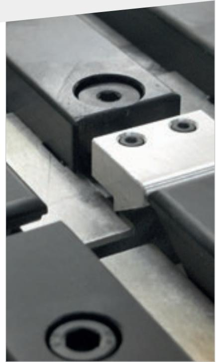
Cutting line closure system, to prevent the longitudinal trim cuts from falling into the machine and fouling the blade path.
