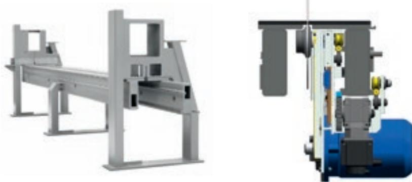
The optimal balancing and weight distribution on the two guides guarantees the total absence of vibrations and perfectly straight cutting action.
