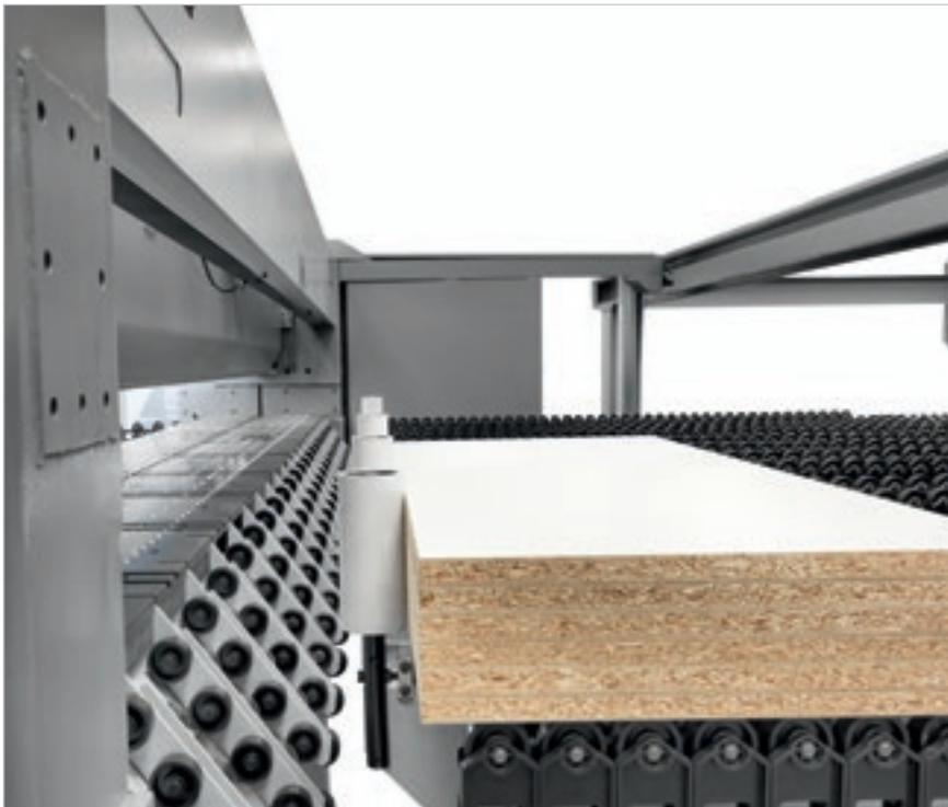
The stacks of strips are selectively transferred to the cross cut area according to the cutting cycle worked out by the Numeric Control.
