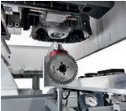
The Pick Up station supports automatic tool-holder rack tooling.
