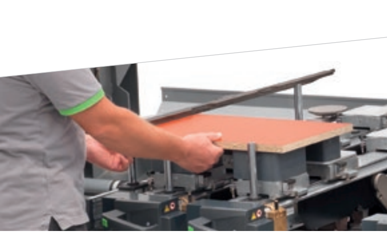
Locking systems based on a vacuum .
