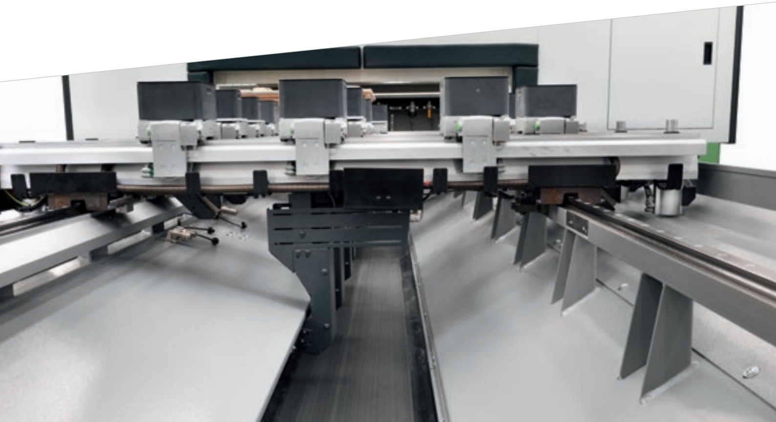
Motorised mat for chip removal.
