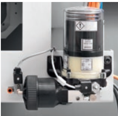
Automatic lubrication boring head BHZ 29 2L.
