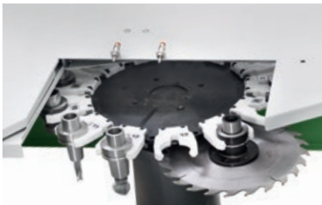
Revolver tool magazine with 13/16 places.
