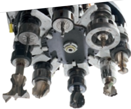
Revolver tool magazine with 8 places.
