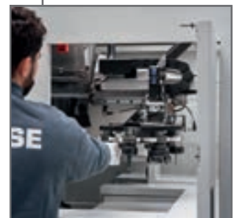
Rear access door to reduce tooling times.
