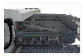
The mechanical arm ensures that the panel is easily inserted and squared.
