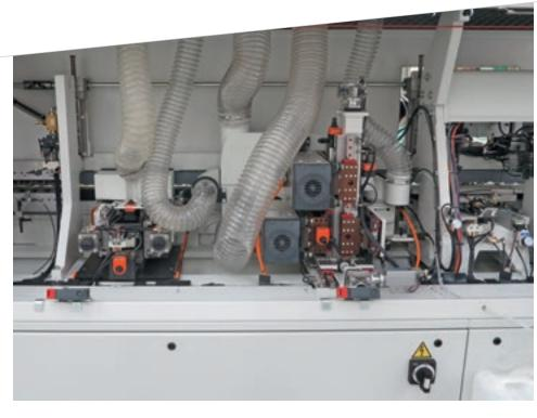
The multi-zone guide system, high precision brushless motor and multiple pressure system drastically reduce the space between panels and increase productivity.
