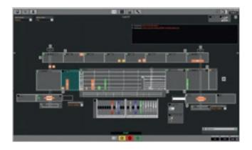
**The line supervisor** controls the flow of material in the Stream B MDS and can see the state of the machine, the position and number of panels and the working processes in REAL TIME.
