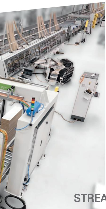
Stream B MDS 2.0 is designed to be operated both automatically and manually. Robots, loaders or any other interlock system can be easily integrated in this version of the machine.
