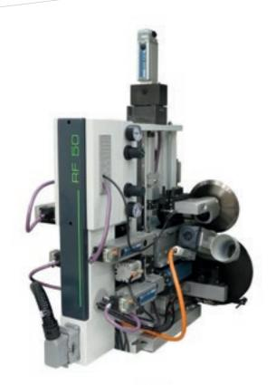
The corner cutting unit and edge scraper are finishing units that guarantee excellent machining repeatability thanks to the real-time management of the panel thickness.
