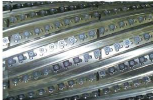
W250/16 is the unit in diameter 250 mm, with 16 sequences of inserts
