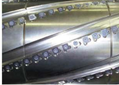
W250/8 is the unit in diameter 250 mm, with 8 sequences of inserts
